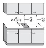
As a general rule there must be a minimum safety distance of at least 30 inches (760 mm) between the top of the appliance and any cabinet above it, ②. The minimum distance of combustible surfaces located above and to the side of the cooktop, ③, is 18" (457 mm).
