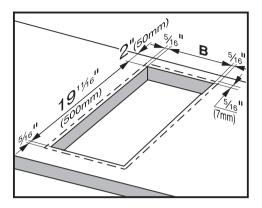
All Miele combisets have the same length and width. Make sure that there is enough room beneath the countertop to allow for the depth of the various appliances. When installing a KM 402 / KM 403 or KM 410 / KM 411 remember to allow clearance for the drain valve that will be located in the cabinet beneath the appliances.
