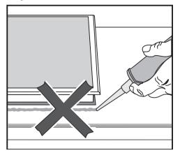
The cooktop must not be permanently sealed into the countertop when installed. The sealing strip under the edge of the cooktop provides a sufficient seal for the countertop.
