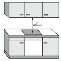
As a general rule there must be a safety distance of at least 30" (760 mm) between the appliance and any objects above it, e.g. cabinetry, venting hood, etc. If the manufacturer of these items states a different figure, always adhere to the greater distance. These measurements should be given in their operating and installation instructions.
