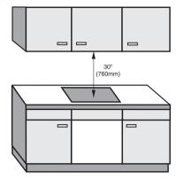
As a general rule there must be a safety distance of at least 30" (760 mm) between the appliance and any objects above it, e.g. cabinetry, venting hood, etc. If the manufacturer of these items states a different figure, always adhere to the greater distance. Their measurements should be given in their operating and installation instructions.
