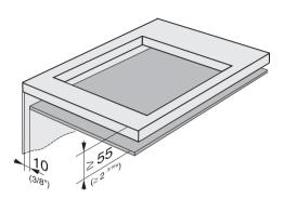
The cooktop bottom must be installed in such a way that the bottom is shielded and cannot be touched.
