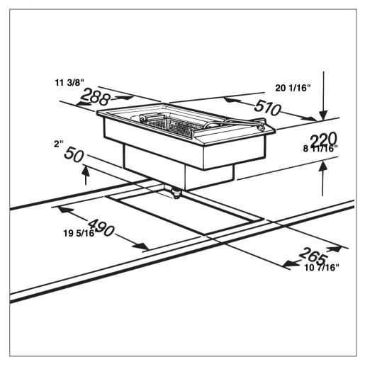
This appliance is classified as "Y" class for heat protection. There may be a wall at the rear and a wall or tall cabinet at one side. On the other side, however, no cabinet or wall must stand higher than the appliance.
