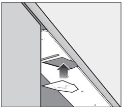
■ Press the reflector panel into the plastic holder in the cover plate.
