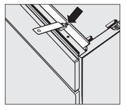
■ Fit the securing pieces into the slots on both the left and right hand sides.
