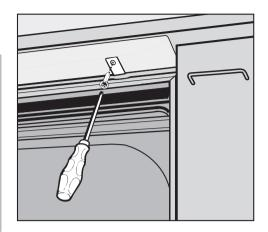
Screw the countersunk screws (3.9 x 22) supplied upwards through the securing pieces on the left and right hand sides into the work surface to secure the dishwasher.
