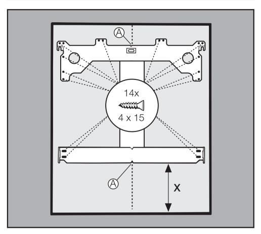
There are notches on the fixing bracket, marked (A) in the illustration.
