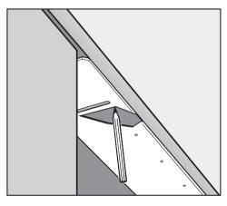
Align the cover plate to the front edge of the worktop in the **middle** of the niche. Draw around the cut-out for the plastic holder. If the worktop has a **very rounded** edge, pull the cover plate further forward so that the reflector panel is visible later. Stick the doublesided adhesive strip supplied onto the back of the plastic holder.
