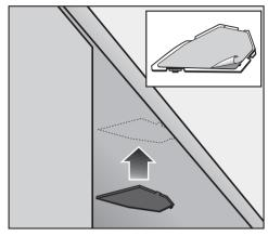
Remove the protective foil from the adhesive strip and stick the holder to the underside of the worktop at the marked position.
