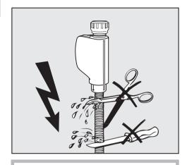
↑ The water inlet hose must not be shortened or damaged in any way, (see illustration).
