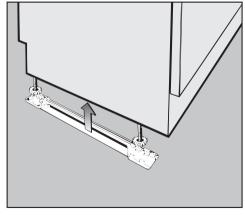
■ Fit the slides - with the ratchet at the rear - under the screw feet.
