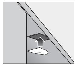
Press the reflector panel into the plastic holder.
