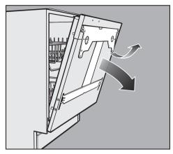
Hold one corner of the upper fixing bracket and pull towards you (small arrow).
