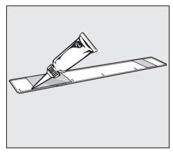
Squeeze sealant from the tube supplied all the way along the hollow moulding in the cover plate.
