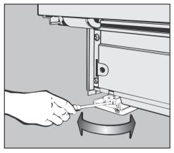
■ Adjust the <u>front screw feet</u> manually or with a flat blade screwdriver.
