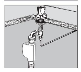
If the stopcock is situated in the worktop, a special angle connector can be ordered from the Miele Spare Parts Dept. (Part No. 04 274 820).
