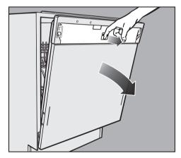
Insert your finger into the T-shaped opening in the door opener and pull the door open.
