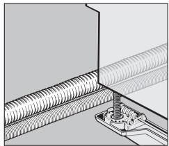
Push the dishwasher right back into the recess. Ensure that the drain hose, inlet hose and the electric cable are laid to reach the connection point without any kinks.
