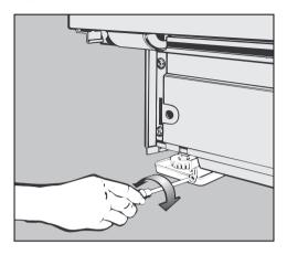
■ Use a TORX T20 screwdriver to adjust the <u>rear screw feet</u> to the required height.
