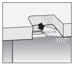
When the dishwasher is built-in, the left hand side of the reflector panel must be sited above the in-operation light in the dishwasher control panel.
