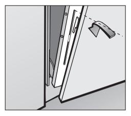
Hang the door front so that the lower lugs of the fixing bracket fit into the lower slits of the dishwasher outer door panel, and draw slightly upwards.
