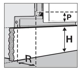
The height (**H**) of the plinth facia in front of the dishwasher depends on the plinth return (**R**) and how much the door front extends below the dishwasher door (**P**).
