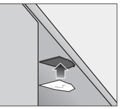
Line up the reflector with the tracing and press into place.
