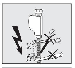
WARNING - Electrical Hazard Do not cut the intake hose. If the hose is cut, the dishwasher will not work. There will be a water leak and you could be injured. If the hose is too long, coil it neatly and place it behind the machine.
