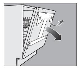
Gently pull on the upper portion of the mounting bracket until the door latch releases (small arrow). Without the mounting bracket in place:
