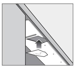
Press the optic indicator reflector in place.
