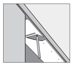
With the reflector cut out left and frontward, align the steam deflector with the front edge of the counter. Trace the outline of the reflector onto the underside of the counter with a pencil.
