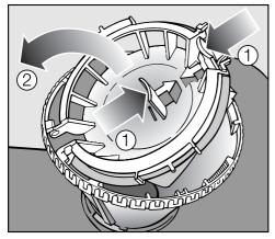
To clean the inside of the filter, the flap must be opened:
