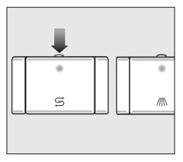
Press the button on the top of the salt reservoir in the direction of the arrow.
