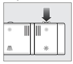
■ Press the button on the lid of the rinse aid reservoir in the direction of the arrow until the flap springs open.
