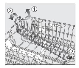
■ To remove an insert, gently pull up on the handle.
