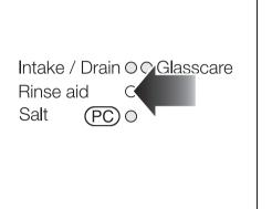
The rinse aid indicator on the control panel will light when the rinse aid reservoir needs refilling.
