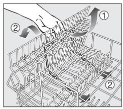
■ To remove an insert, gently pull up on the handle.
