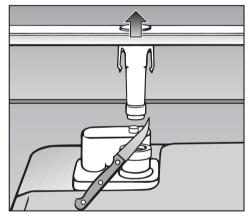
■ Cut off the vent cap located at the right rear of the triple filter system, as illustrated.
