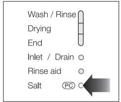
■ Fill the salt reservoir with dishwasher salt when the salt indicator light comes on. (If it comes on during a programme, wait until the end of the programme).
