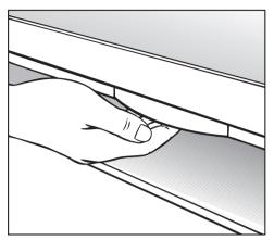
■ Press the release catch inside the door grip and pull forward.
