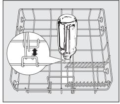
■ Place the bottle holder as shown in the bottom basket. If placed anywhere else, water will not be able to access the bottle properly, and cleaning results will be impaired.
