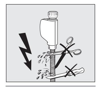
⚠ Do not cut the intake hose. It contains electrical wiring. If the hose is cut, the dishwasher will not work. There will be a water leak and you could be injured. If the hose is too long, coil it neatly and place it behind the machine.
