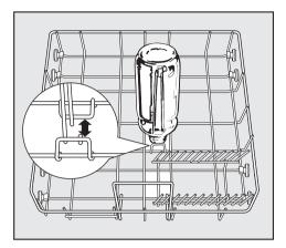
The vase/bottle holder, e.g. for vases and baby bottles, can be inserted into the lower basket as shown in the illustration.
