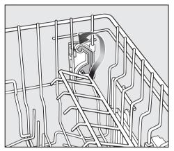
■ Pull the cup rack upwards and let it engage at the desired height.
