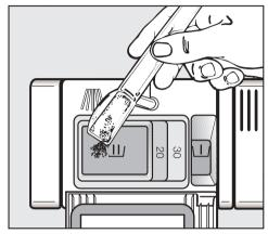
The horizontal marks in compartment II indicate the levels of approximately 1 ¼ and 2 tablespoons (20 and 30 ml) respectively. Compartment I holds a maximum of 2 teaspoons (10 ml).
