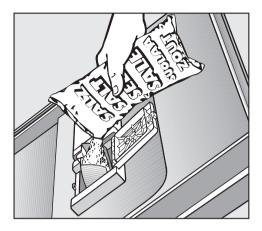
Carefully fill with salt until water runs out. The salt container holds approx.
