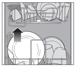
The guide at the front of the upper basket determines the maximum height for items placed in the lower basket so that the middle spray arm is not blocked.
