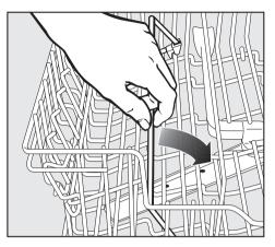
To allow water to run off the bottom of coffee mugs, place them slanted on top of the coffee bar. The bar can also be used to separate two rows of glasses. To stack wide items, flip the bar to the right.
