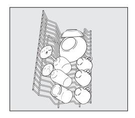
Hook the PlateGuard Plus insert into the left half of the lower basket, the area marked in white.
