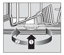
■ Lift up the <u>middle</u> spray arm, ①, to engage the ratchet and unscrew the spray arm, ②.
