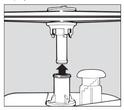
■ First remove the bottom basket and then pull the **lower** spray arm off.
