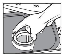
To unscrew the micro-fine filter, take hold of the two lugs and turn twice in an anti-clockwise direction,
