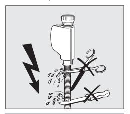
The inlet hose must <u>not</u> be shortened or damaged in any way (see illustration).
