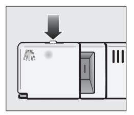
Press the opening catch on the container forwards (see arrow). The flap will spring open. (The flap is always open at the end of a programme).
