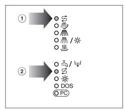
When the salt reservoir is empty the S indicator light (2) comes on to remind you to fill the reservoir.
