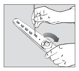
Particles in the <u>lower</u> spray arm are easier to rinse out if the cap is first opened.
