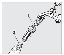
Clean the large area filter (1) and fine filter (2), and replace with new filters if necessary.
