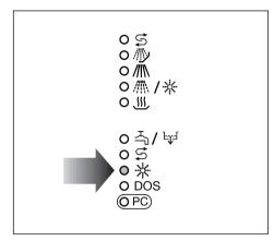
If the \* Add rinsing agent indicator light on the control panel comes on, the rinsing agent reservoir must be refilled.
