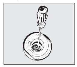
The dosage adjuster in both openings has settings from 1-6 (1-6 ml). It is set to "2" (4 ml) at the factory.
