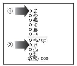
When the salt reservoir is empty the  $\preceq$  indicator light ② comes on to remind you to fill the reservoir.
