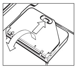
Press the opening catch on the dispenser (see arrow) forwards. The lid will spring open. (The lid is always open at the end of a programme).
