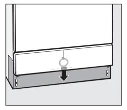
■ The emergency release cable is located at the bottom of the machine behind the service panel. Pull it downwards to open the door.
