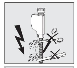
The inlet hoses must <u>not</u> be shortened or damaged in any way (see illustration).
