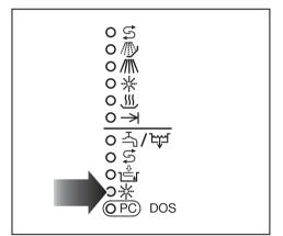
The reservoirs must be filled with rinsing agent when the \* indicator light comes on.
