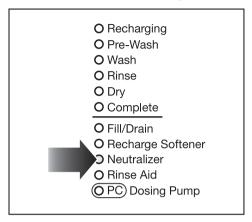
■ When the "Neutralizer" indicator light comes on, it is important to promptly refill or exchange the neutralizer container.
