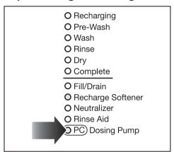
■ When the "OPC Dosing Pump" indicator comes on, it is important to promptly refill or exchange the detergent container.
