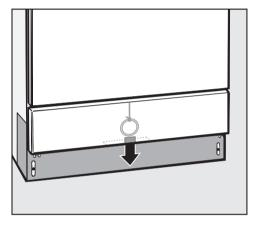
Locate the ring for the emergency release cable (at the bottom of the machine, behind the service panel), and pull the ring downward to open the door. Before using the machine for the first time, the water softener should be programmed. The water needs to be softened to avoid calcium deposits on the items being cleaned and in the machine itself.
