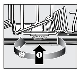
■ Lift up the <u>middle</u> spray arm ①, to engage the ratchet and unscrew the spray arm ②. Remove the lower basket.
