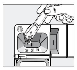
Fill the dispenser with 1 ½ tablespoons (25 ml) of powder detergent, or place a detergent tablet into compartment II.  Close the cover. The cover will always be open at the end of a wash program (except "Rinse & Hold").
