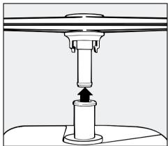
Pull the <u>lower</u> spray arm firmly upwards to remove.
