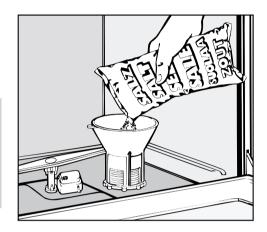
Before adding salt for the first time, fill the reservoir with approximately 1 quart (1 l) of water.
