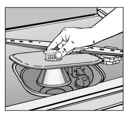
Lift the combination filter out of the machine. Remove any coarse particles and rinse under running water. A nylon brush can be used.
