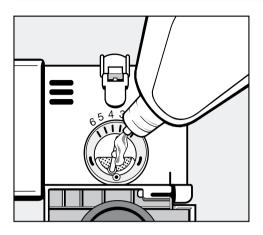
Pour liquid rinse aid into the reservoir until it is visible on the surface of the screen. Do not refill until the "Rinse Aid" indicator lights.
