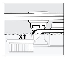
The water level is correct when dimension "X" is at least 1/8 "(4 mm).
