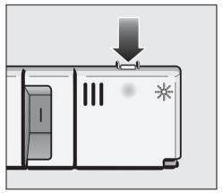
Press the button of the rinse aid reservoir flap in the direction of the arrow until the flap springs open.
