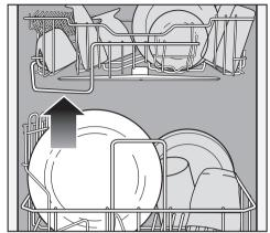
The guide at the front of the upper basket shows the maximum height for items placed in the lower basket so that the middle spray arm is not blocked.
