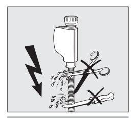
⚠ The inlet hose must **not** be shortened or damaged in any way (see illustration).
