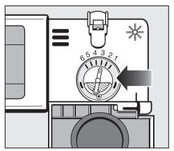
The dosage selector has settings from 1-6. It is factory set to the recommended setting "3" (3 ml). Approx. 3 ml of rinse aid are used per program.
