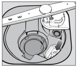
The drain pump is located under the non-return valve (see arrow).
