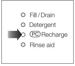
After the reservoir has been filled, the water softener is automatically reactivated the next time the dishwasher is run. The salt indicator may still light during this process. It will go out once the salt concentration has reached the correct level.
