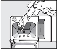
The horizontal marks in Compartment II indicate levels of approximately 20, 25 and 30 ml respectively.
