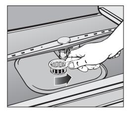
■ Turn the handle counterclockwise to release the triple filter.
