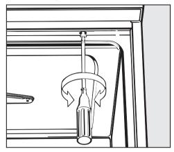
If necessary, remove the lid from the machine to make installation possible.
