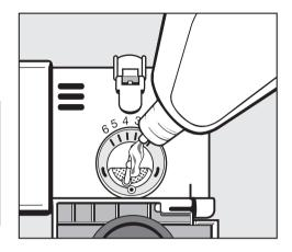
Add rinse aid until it is visible on the surface of the filter in the opening.
