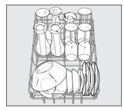
The lower basket glassware insert is designed for washing tall glasses. Tall glasses are held securely by the vertical supports.
