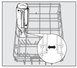
The bottle holder is designed for washing slim items e.g. milk or baby bottles. For best results place the bottle holder into the lower basket as shown. The spray jets can reach the inside of the bottle in this position.
