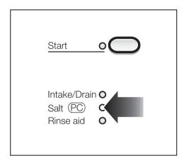
After the reservoir has been filled, the water softener is automatically reactivated the next time the dishwasher is started. The "Salt" indicator will be lit during this process.
