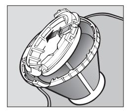
To clean the underside of the filter, the flap must be opened:
