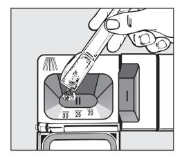
The horizontal marks in Compartment II indicate levels of approximately 1 <sup>1</sup>/<sub>4</sub>, 1 <sup>3</sup>/<sub>4</sub> and 2 tablespoons (20, 25 and 30 ml) respectively.
