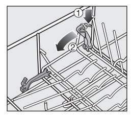
Hook the foldable spike insert into the back right corner of the lower basket, the area marked in white.
