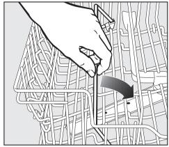
To allow water to run off the bottom of coffee mugs, place slanted on top of the coffee bar. The bar can also be used to separate two rows of glasses. To stack wide items, flip the bar to the right.
