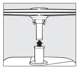
■ Pull the <u>lower</u> spray arm firmly upwards to remove.
