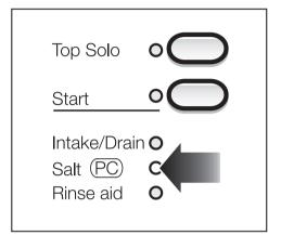
After the reservoir has been filled, the water softener is automatically reactivated the next time the dishwasher is started. The "Salt" indicator will be lit during this process.
