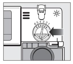
The dosage selector is preset to 3. This dispenses approximately 3 ml of rinse aid per program. It can be adjusted from 1 to 6.
