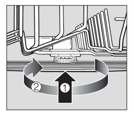
Lift up the <u>middle</u> spray arm, ①, to engage the ratchet and unscrew the spray arm, ②. Remove the lower basket.
