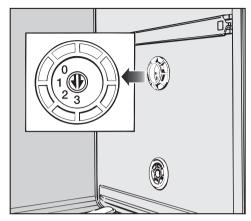
Use a coin or screwdriver to adjust the water hardness selector. There is a click as each setting is reached.
