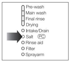
After the reservoir has been filled, the water softener is automatically reactivated the next time the dishwasher is started. The "Softener" indicator will light during this process.
