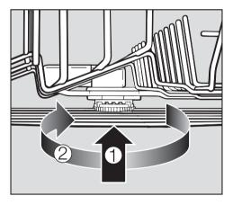
Lift up the <u>middle</u> spray arm, 1, to engage the ratchet and unscrew the spray arm, 2. Remove the lower basket.
