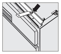
Insert the tab of each bracket into the guide holes on the top of the dishwasher.
