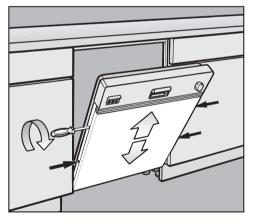
Open the dishwasher door slightly. If the locking screws on the edge of the dishwasher door can not be reached, the dishwasher will have to be pulled out of its opening a few inches.
