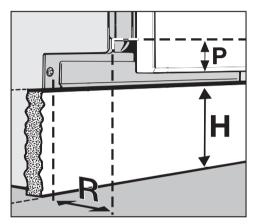
The door panel overhang (**P**), and toekick depth of recess (**R**), determine the maximum dishwasher toekick height (**H**).
