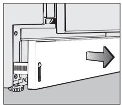
Screw the toekick onto the installed brackets, with the cutting lines towards the top, and pull out evenly and slowly until it aligns with the toekick of the adjoining cabinets.
