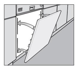
Attach the panel to the dishwasher by lining up the bracket tabs with the slots on the door.
