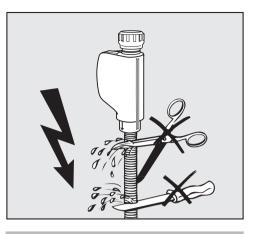
Do not cut the intake hose. If the hose is cut, the dishwasher will not work. There will be a water leak and you could be injured. If the hose is too long, coil it neatly and place it behind the machine.
