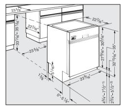
Machine heights of 35" - 37" (889 - 940 mm) can be obtained if the supplied legs are removed and extended legs are attached. Contact the Miele Technical Service Department for the appropriate legs (part # 02 702 601).
