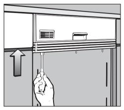
Using an 8 mm socket, turn the nut clockwise or counterclockwise until the filler strips line up with the drawer line.
