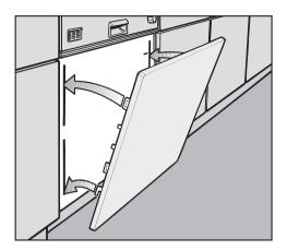
Attach the panel to the dishwasher by aligning the bracket tabs with the slots on the door.
