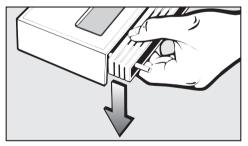
To remove the filler strips from the control panel, place the panel printed side up, and gently push down near the bottom of the control panel. This will release the mounting bolts from their slots.  After adjusting the control panel height, cut off the plastic screw excess.
