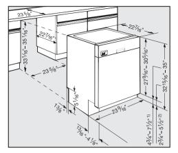
Machine heights between 35" and 37" (889 - 940 mm) can be obtained if the supplied legs are removed and extended legs are attached. Please contact the Miele Technical Service Department for the appropriate legs (part # 02 702 601).
