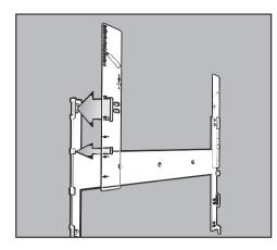
Place a template on each end of the mounting bracket as shown, making sure the rule marks face the outside of the bracket.
