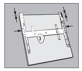
Tape the bracket to the door panel to hold it in place while the mounting holes are drilled.
