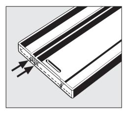
The rear of the toekick has two cutting lines.
