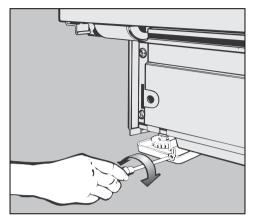
The rear leveling legs can be adjusted with a T20 Torx screwdriver by turning the screws at the front of the slide skis.
