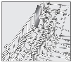
Slide the glass rack to the desired height until the catches click into place at the top and rest on the bottom
