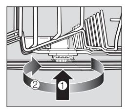
■ Lift up the **middle** spray arm, ①, to engage the ratchet and unscrew the spray arm, ②.
