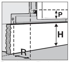
The panel overhang  $(\mathbf{P})$ , and toekick depth of recess  $(\mathbf{R})$ , determine the maximum dishwasher toekick height  $(\mathbf{H})$ .
