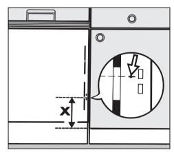
Measure the distance (X) between the lower mounting hole on the dishwasher front door (see inset arrow) and the lower edge of the neighboring cabinet door.
