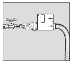
If the standard 3/8" copper plumbing for a dishwasher already exists with a compression fitting and valve as pictured:
