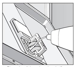
Close the dishwasher door halfway and pour liquid rinse aid into the storage container until it is visible on the surface of the screen. Do not add aid until the "Rinse aid" indicator lamp comes on.
