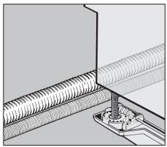
Push the machine into the opening, making sure the electrical cable and hoses can reach their connection points without being kinked.
