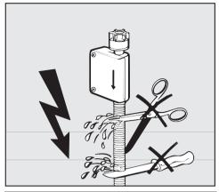
Do not, under any circumstances, cut the intake hose. If the hose is cut, the dishwasher will not work, you will have a water leak and you could be injured. If the hose is too long, coil it neatly and place it behind the machine.
