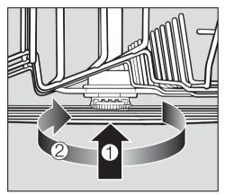
■ To remove the <u>middle</u> spray arm located beneath the upper basket, gently push upwards until it engages in the ratchet ①, then unscrew it ②.
