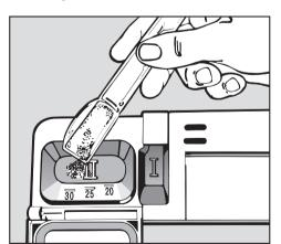
Close the cover. The cover will always be open at the end of a wash program (excluding the RINSE & HOLD program). Generally, filling the dispenser with detergent will be sufficient to ensure thorough cleaning. If dishes are extra dirty, or if the soil has been allowed to dry on the dishes before washing, a program utilizing a prewash cycle should be selected. In this case, extra detergent can be added to the small compartment labeled ( I ) in the center of the dispenser.
