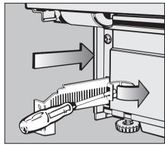
■ To adjust the depth (recess) of the toekick, release the tension on the spring clips as shown, and push the mounting brackets in as far as possible.
