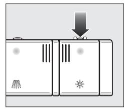
■ Press the button on the lid of the rinse aid reservoir in the direction of the arrow. The flap will spring open.
