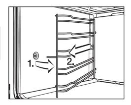
■ Pull the runners out of holder (1) at the front of the oven and then pull them out of the oven (2).
