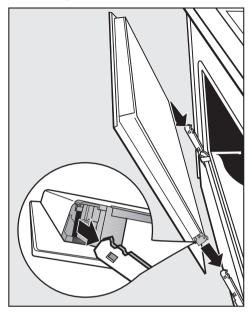
■ Hold the door securely at both sides and carefully fit it back into the hinge retainers.
