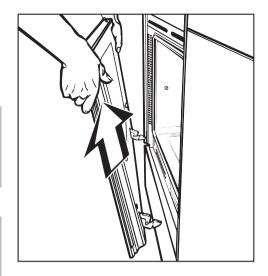
■ Lift the door up until it is nearly in the closed position. The hinges will automatically swing out in this position, then remove the door.
