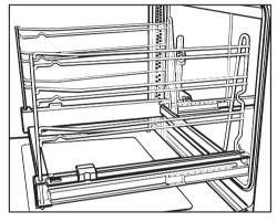
The telescopic carriage with 4 levels of runners can be drawn right out of the oven.
