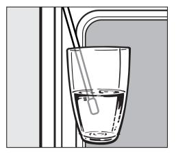
■ Hold a container with the quantity of water specified under the tube as shown. Start the water intake process with "OK".
