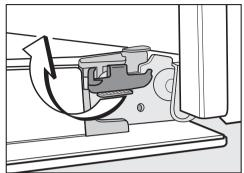
Flip both locking clamps back up as far as they will go into a horizontal position.
