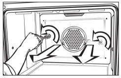
Remove the screws in the back panel and take it out.
