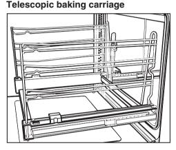
The telescopic baking carriage has four shelf levels and can be drawn right out of the oven, giving a good overview of cooking in progress.
