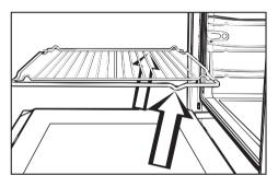
When pushing the tray and rack back in, always ensure that the safety notches are at the rear of the oven (see illustration).
