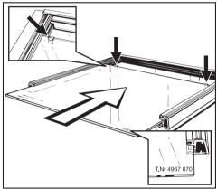
Push the middle pane into the frame almost to the end. The material (M-) number printed on the pane must be legible in the bottom right hand corner (see illustration). Fit the sealing strip into position, then push the pane in as far as it will go.
