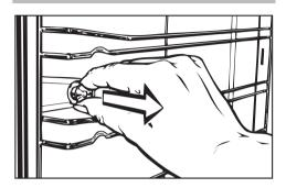
■ Pull on the fixing knob to release it.
