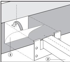
■ Place the supplied spring clips ① and the support bars ② at the marked positions as shown above, by laying them on the upper edge of the cut-out and then securing them with the ¹/<sub>8</sub>" x 1" (3.5 x 25 mm) screws (supplied).
