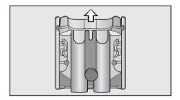
■ Turn the cover around, slide the insert upward and out, and clean both parts thoroughly.
