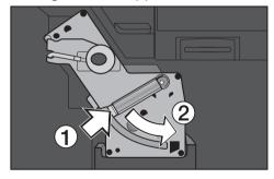
■ Press the light colored button on the brew unit handle, ①, and turn the handle to the right, ②, to lock it into place.
