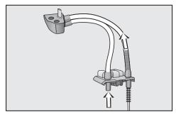
■ Insert the brush into the milk hoses one after the other from below. Push the brush back and forth to the end until there is no more no milk residue in the hoses.
