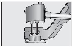
■ Push the retainer with the plug onto the cover as shown. Make sure that the retainer is sitting properly on the cover.
