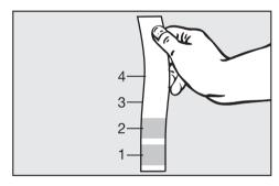
■ Place the test strip under your kitchen tap for a second and shake off any remaining water. The result is visible in about 1 minute.
