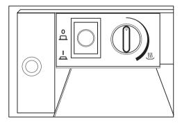
The controls consist of a temperature dial and an On/Off switch. These are only visible when the drawer is open. When the drawer is closed, you can tell when the appliance is switched on because the On/Off switch illuminates through a hole in the front of the drawer.
