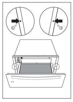
Open the drawer and fix the appliance with the two supplied screws at the side panels of the cabinet. The installation kit contains 3 metal strips with adhesive on the back side.
