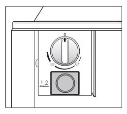
The controls consist of the temperature selector and the On/Off button. They are only visible when the drawer is open.
