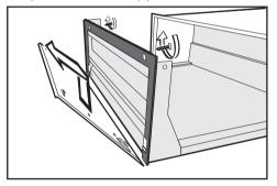
■ Pre-drill the custom front panel (see illustration). Ø 3/8" (10 mm), t = 3/8" (10 mm)
