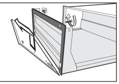
Pre-drill the custom front panel (see illustration). Ø 3/8" (10 mm), t = 3/8" (10 mm)
