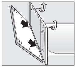
8 Hook the panels into the bottom on and secure at the top with two screws making sure the seal is seated correctly.
