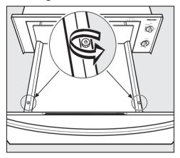
■ Pull the drawer completely out and loosen the nuts.
