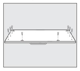
Screw the removed panel to the custom panel with the eight screws.
