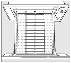
■ Insert the rack into the slots of the rear wall in the drawer and then slide the front of the rack into position.
