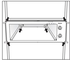
■ Secure the casing in the cabinetry with the six screws.
