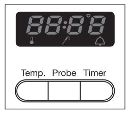
Each push button has a matching symbol in the oven display.
