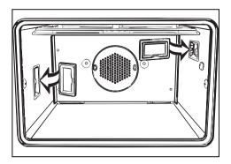
Press the lamp back into the sidewall of the oven and reinsert the cover.
