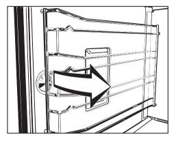
Pull on the fastener to release the runner.
