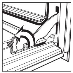
Flip up the locking clamps on each door hinge.
