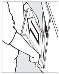
Grip the sides of the door and lift until the hinges disengage. Remove the door.
