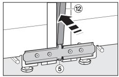
■ Position the long stainless steel trim ② in the gap, making sure that it is located above bracket ⑤.
