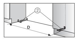
The distance "**D**" between the anti-tip brackets ② is the width of the appliance.
