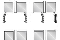
The minimum thickness of the partition is  $\frac{5}{8}$  (16 mm).
